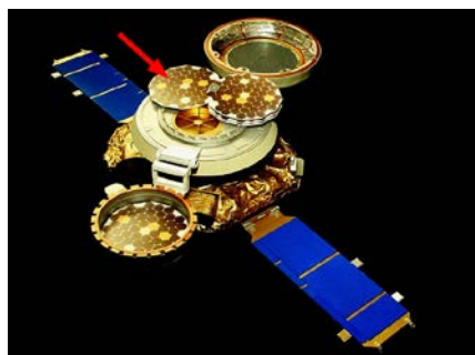
Fig. 1 One of 3 solar wind regime collector arrays unshaded in solar wind capture configuration (red arrow). Onboard algorithms determined which of the 3 arrays was placed in unshaded configuration [1].
