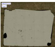
Fig. 6. Example Coronal Hole sample 30985, 11mm x 8 mm. Float zone silicon.
